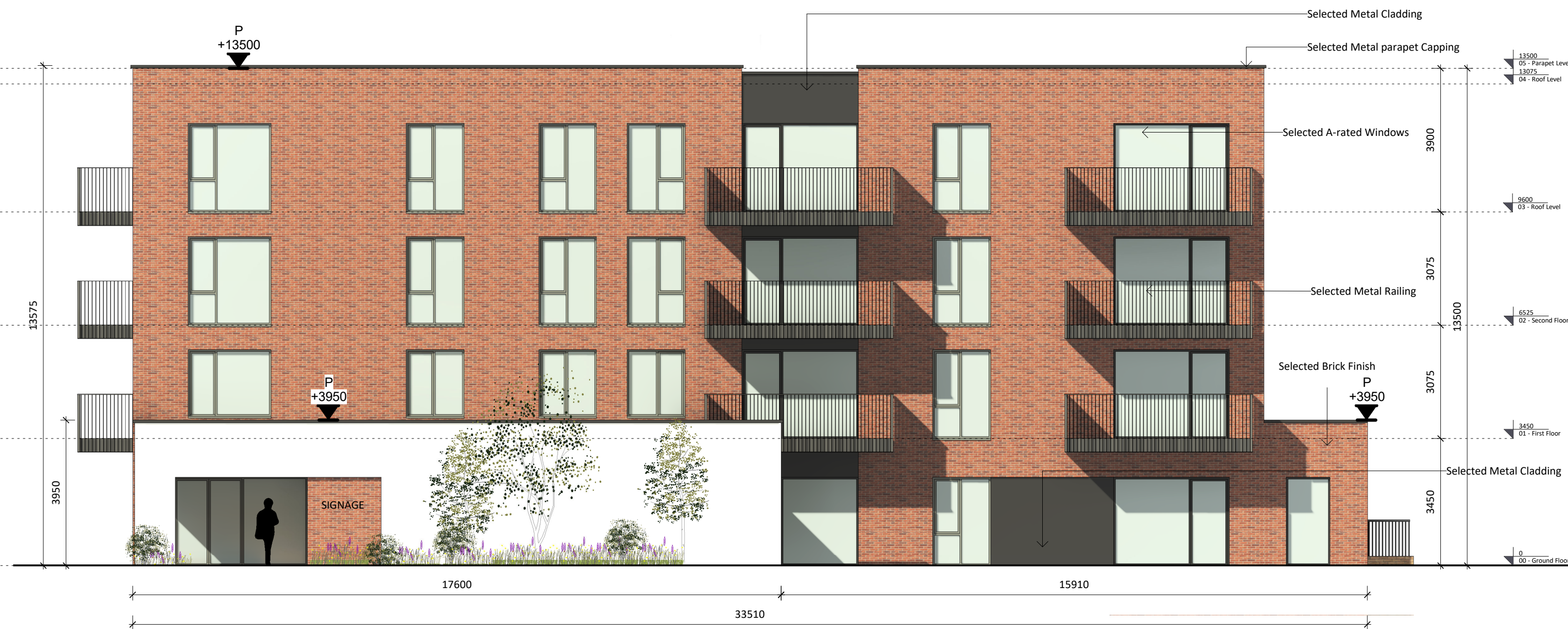
④ Block A - Rear Elevation 1:100
