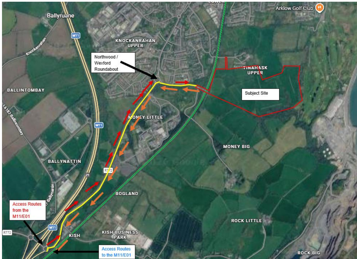
Figure 2: Construction Access Route
