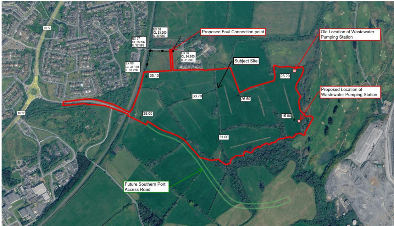
Figure 3-2: Proposed Amendment to Foul Pumping Station Location
