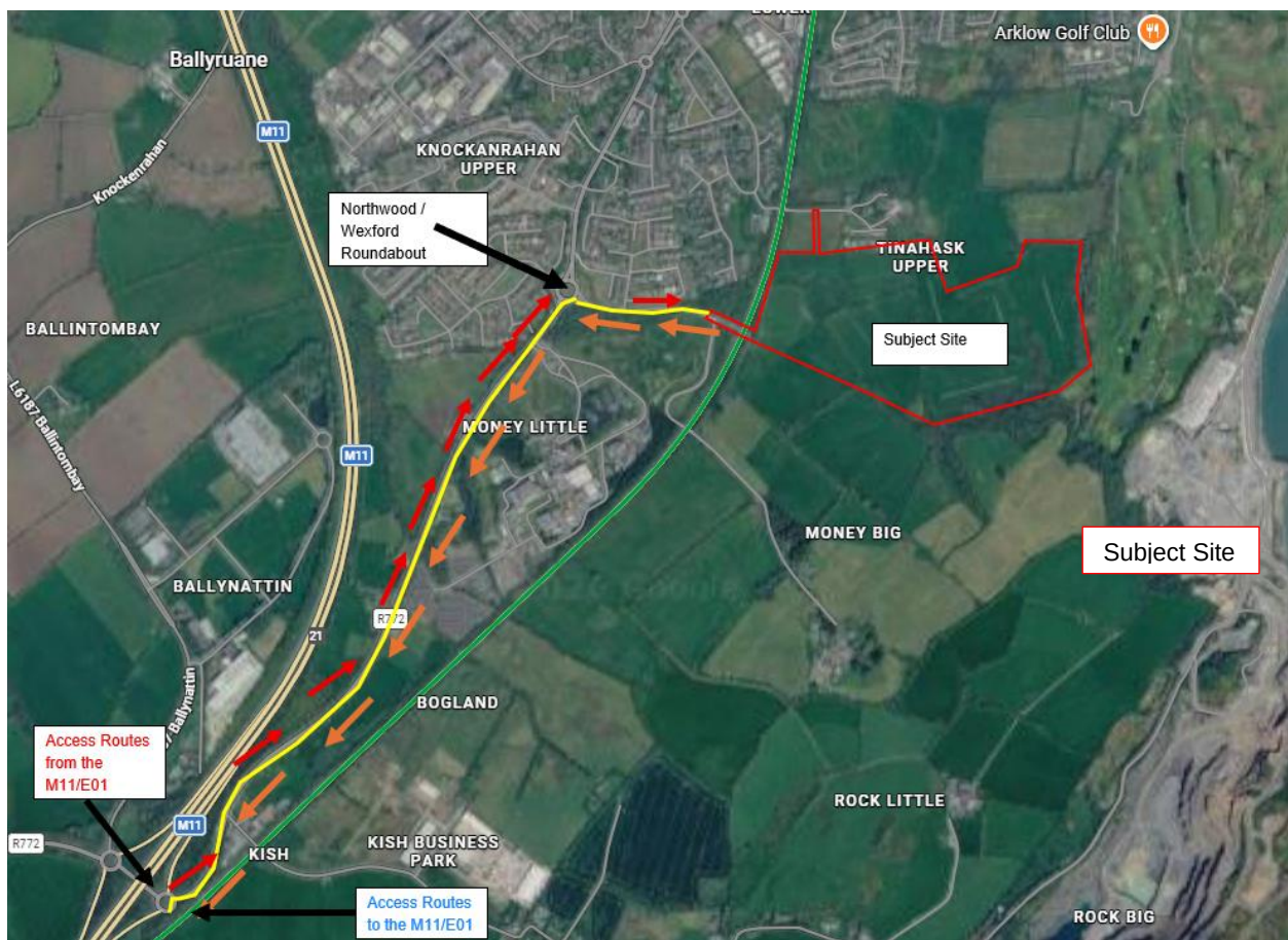
Figure 3-2: Construction Traffic Routes to/from Proposed Site Compound
